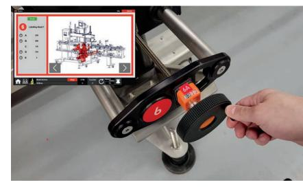
in the screen to the corresponding color and letter on your machine. And when done, that recipe is saved in the HMI and ready to be recalled at the push of a button for a ridiculously quick and easy replication.
