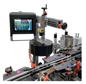
Professional grade cameras or sensors married to servo motor-driven belt systems rotate both round or square containers. Available integrated into a powerful NITA Labeler or as a convenient Stand-Alone Orientation System when a label application is not needed.
