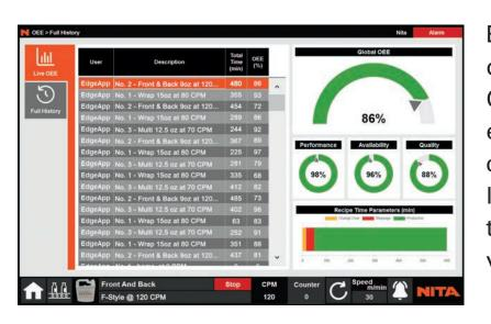
Every NITA includes a live S.C.A.D.A. dashboard allowing for real time O.E.E. data and other production efficiencies like uptime, downtime, changeover times and container and label usage to be viewed right from the comfort of your Panel PC HMI or via OPC/UA connectivity.
