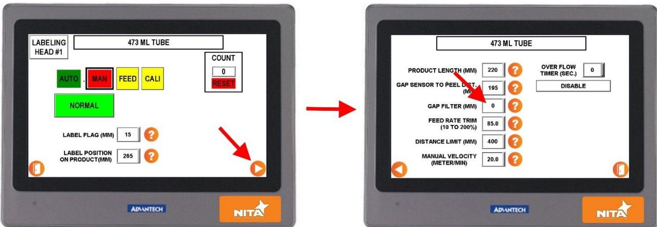
On this screen you will enter the label length to be ignored by the sensor. The example above shows us that the proper value to be entered is between 135 & 168 mm a recommended value to be entered in the HMI screen, for this application would be 152mm.
