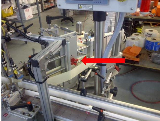
Secondly, the coder can be rotated 90 degrees. This will be used to change the orientation of the code on the label. To change the orientation, simply loosen the rotation adjustment handle and rotate the Coder 90 degrees. When the coder reaches its new position, you will hear (and feel) a little “click”, meaning that it is well seated in its rack mount.
