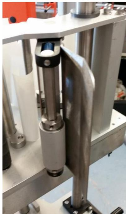
8) Wind the label stock on the re-winder and lock it in place with the u-shaped hook.
