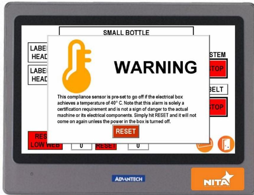
In accordance to the UL73 and CSA C22.2 68 certification norms, an alarm will sound when the internal temperature of the electrical panel reaches 40 C or 104 F. The system will not stop. You simply have to press RESET to remove this alarm. The alarm will not reappear for as long as the machine stays ON. NOTE: please make sure that the vent traps are clean and dust free to ensure proper air circulation within the box.
