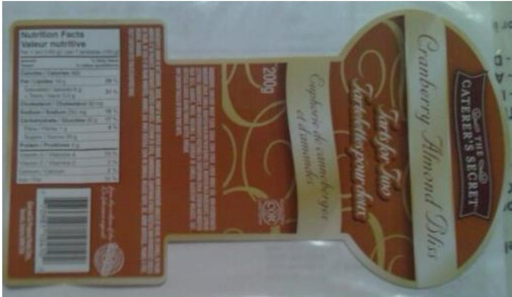
On this example we can clearly see that the signal from the gap sensor would get triggered by two zones of the same label. This will cause two feed triggers for the same label when in fact there is only one label to be fed. To avoid this double feed... **you must adjust** the "GAP FILTER MM" setting which is located in the OFFSET SCREEN (as demonstrated here) This setting is present for each label head on the system (when equipped by multiple labellers).
